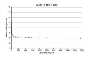
Novec fluorosurfactant FC-4434 is very efficient at reducing the surface tension in aqueous coating systems.
